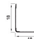
KST-ZH032C Weight: 0.041kg/m
