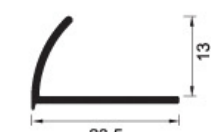
KST-LC22 Weight: 0.113kg/m
