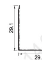
KST-2000-ZH033P Weight: 0.08kg/m
